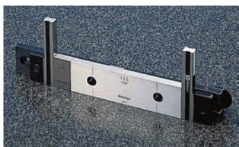
Use of B-type connectors in gage construction
