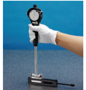
Setting a bore gage using a holder with the pair of Type I half-round jaws arranged as flat contact surfaces
